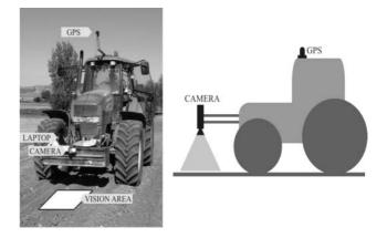
Fig. 1. Global image of the system installed in the tractor. The GPS receiver is placed up. The camera and the laptop computer are in front of the tractor wheels. The camera is focused to the working area. Photographs are taken maintaining the distance constant between the camera and the ground. A long wire connects the GPS to the laptop
