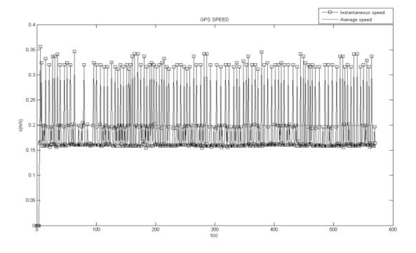
Fig. 9. Instantaneous and average speed with GPS while the machine vision was processing
