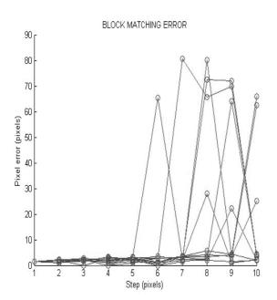
Fig. 4. Block matching machine vision calibration: error distance in pixels vs step. X-axis is the block step search in block matching. Y-axis: error in pixels between the real block position and the position determined by machine vision
