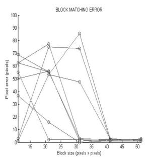
Fig. 5. Block matching machine vision calibration: error distance in pixels vs block size. X-axis is the block size in block matching. Y-axis: error in pixels between the real block position and the position determined by machine vision
