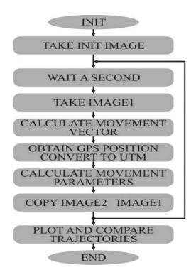
Fig. 2. Block matching and GPS algorithm
