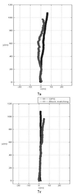
Fig. 7. Trajectories of machine vision system and GPS in (a) Stubble field, (b) Ploughed field, (c) Sunflower stubble field
