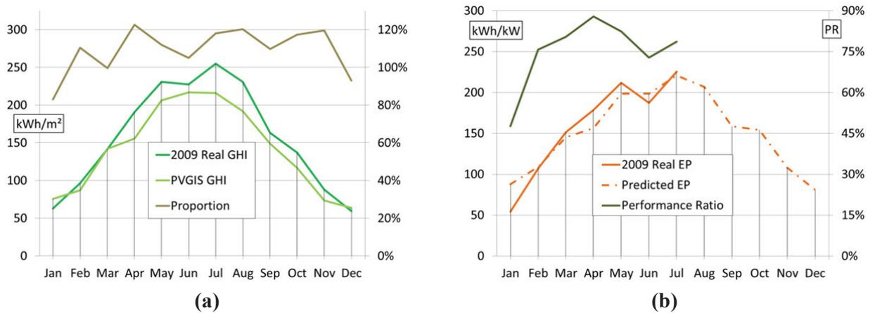
The predicted 2009 monthly EP from January to July from GHI is presented in Table 3 and Figure 5 (b). The predicted EP has been calculated (as in Figure 3 (b)) by estimating DNI from the weather stations, and by assuming a constant monthly PR of 75%. The predicted EP from January to July 2009 is 1111 kWh/kW while the real EP over the same time period is 1117 kWh/kW.
