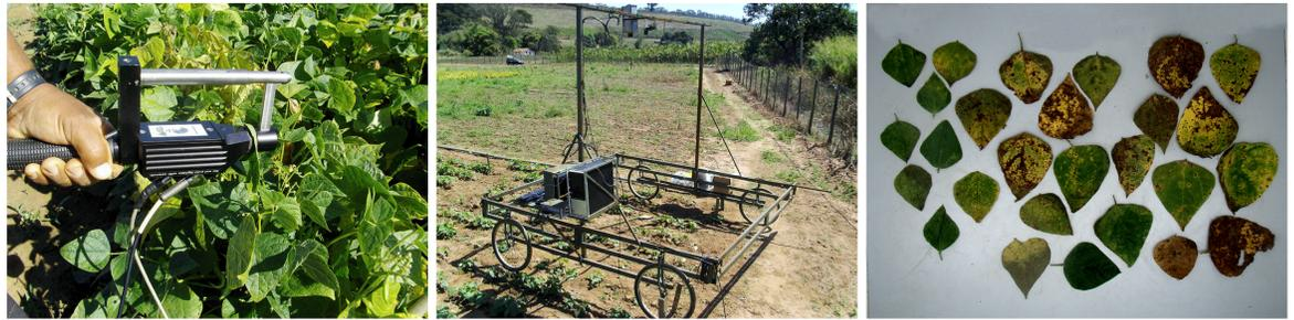
**Fig 1. Representative images of the data acquisition.** (a) spectroradiometer and leaf clip accessory employed to acquire leaf reflectance spectrum, (b) spectroradiometer and platform employed to acquire canopy reflectance, and (c) RGB image of several leaves analyzed.
